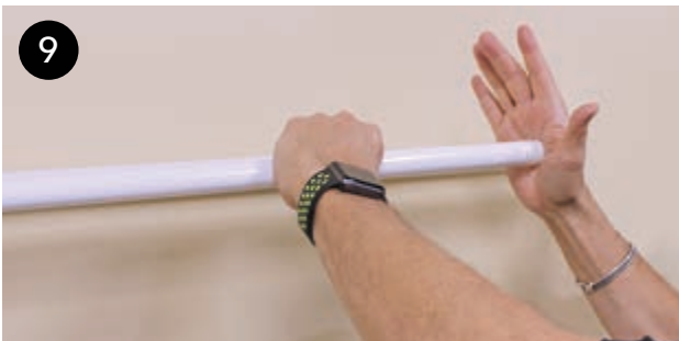
Lock Inner and Outer Tube. Twist the Outer Tube while holding the Inner Tube stationary. Tap the end of the Tube using your palm or hammer/mallet, to fully insert Tube.
